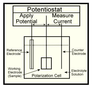
Electrochemical corrosion experiments measure and/or control the potential and current of the oxidation/ reduction reactions. Several types of experiments are possible by manipulating and measuring these two variables.
